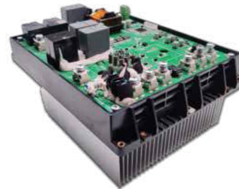
Inverter Compressor Drive
