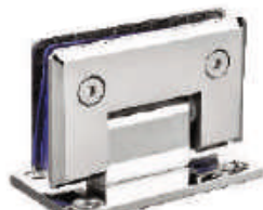
CGC 02 WALL TO GLASS CONNECTOR 90° MAT.: SS 304, FOR 8 TO 12MM
