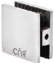
CSSH 13 SQUARE GLASS TO GLASS HINGES 135° (SS 304) FOR 8 TO 12MM
